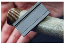
If the pipe scratches with a color that looks like a penny and a magnet doesn't stick, this is a copper pipe. See picture below.
