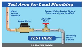
To find the material of your service line, you must use a magnet and a coin. Gently scratch the surface of the pipe with a coin. If the pipe is soft, easily scratched with a silver shine and a magnet doesn't stick, this is a lead pipe.
