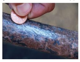
If the pipe scratches with a dull color and a magnet sticks to the pipe, this is a galvanized steel pipe.
